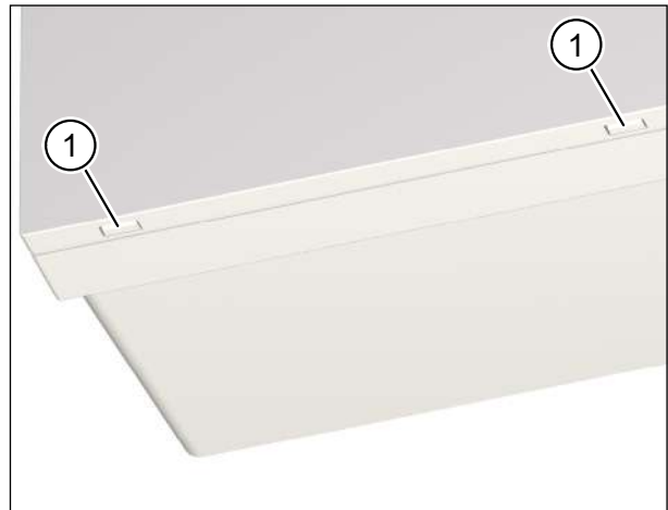
Fig. 34: Removing the unit cover from the ventilation unit
