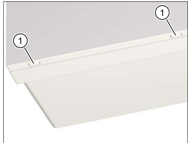
Fig. 25: Removing the unit cover from the ventilation unit
