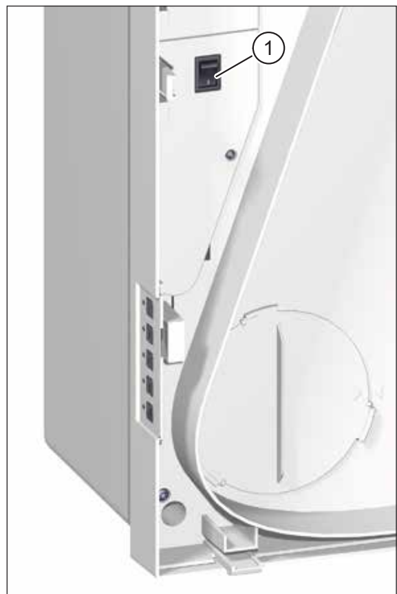
Fig. 13: Mains switch, visible when unit cover is removed
