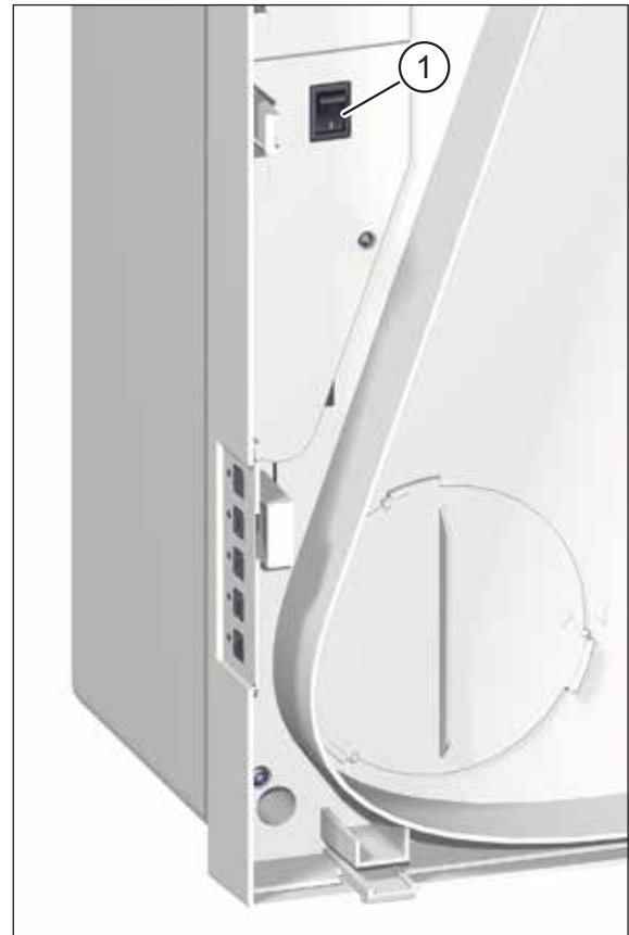
Fig. 12: Mains switch, visible when unit cover is removed
