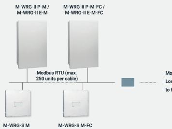
Modbus RTU master (GLT, KNX, Loxone and various other bus systems) to be provided by the customer
