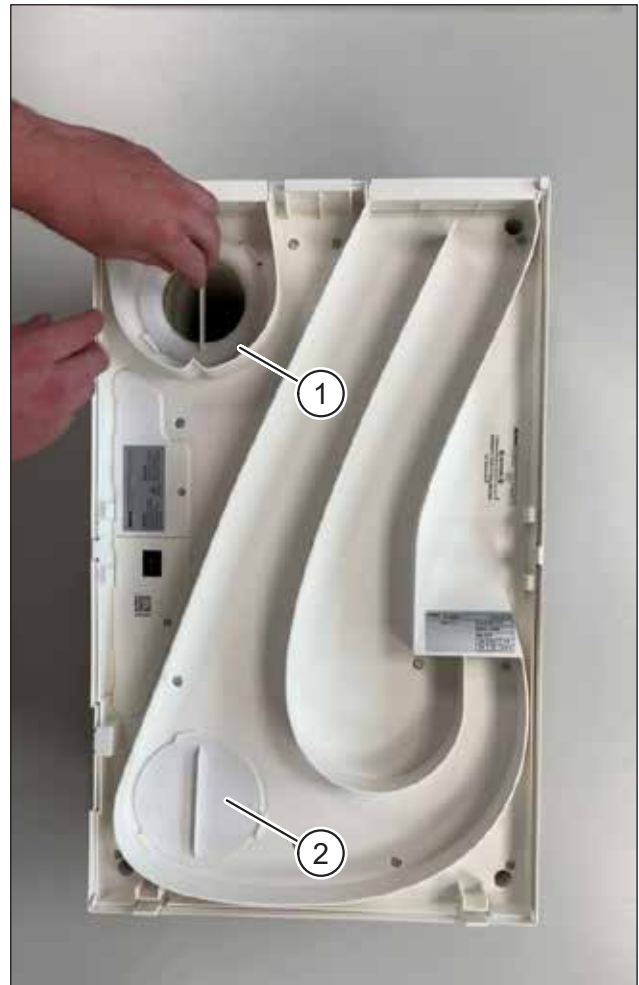
Fig. 2: Remove the air filters
