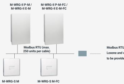
Modbus RTU master (GLT, KNX, Loxone and various other bus systems) to be provided by the customer
