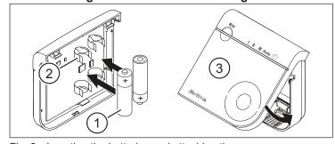
Fig. 3: Inserting the batteries and attaching the cover
