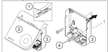
Fig. 2: Fixing the housing to the wall
