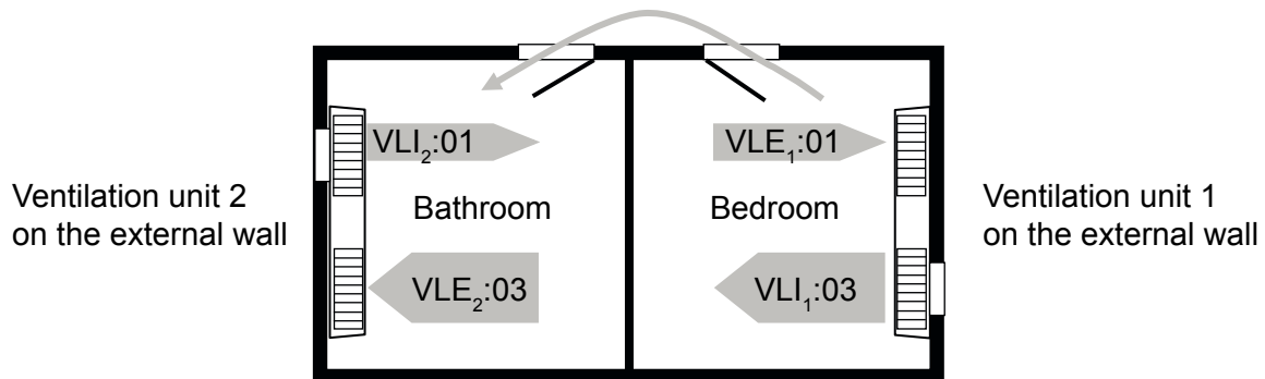
Fig. 16: Cross-ventilation with two ventilation units
