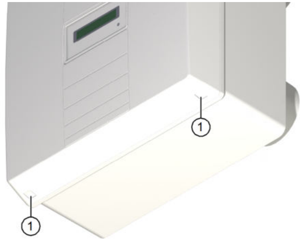
Fig. 17: Remove cover from the ventilation unit
