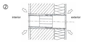
Apply the interior-and-exterior plaster. If you apply an plastering exterior closing, please change before the plaster protection cover against the exterior cover.
