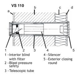
Wall construction: a - interior plaster; b - brickwork; c - insulation; d - exterior plaster;
