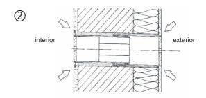
Apply the interior-and-exterior plaster. If you apply an plastering exterior closing, please change before the plaster protection cover against the exterior cover.
