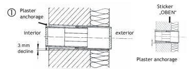
Prepare the wall aperture for the telescopic tube (e.g. by creating a coring ; drill bit 112 mm). Extract the telescopic tube to the required length. Respect for potential overhang of the tube on both sides, to bridge thickness of the plaster. Please note the sticker "Oben" on the plaster anchorage for the interior blind. Please insert the telescopic tube. Caulk it cricular, for examle with fitting foam glue.
