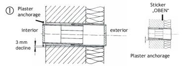
Prepare the wall aperture for the telescopic tube (e.g. by creating a coring; drill bit 112 mm). Extract the telescopic tube to the required length. Respect for potential overhang of the tube on both sides, to bridge thickness of the plaster. Please note the sticker "Oben" on the plaster anchorage for the interior blind. Please insert the telescopic tube. Caulk it cricular, for examle with fitting foam glue.
