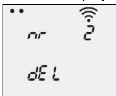
Fig. 14: Disconnect connection to ventilation unit
