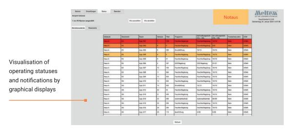
The Meltem Touch Control software can be quickly and easily adapted to various applications. Graphical representation of the room arrangement provides a clear overview and is easy to use.
