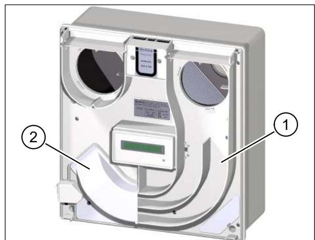
Fig. 11: Supply air hood and intermediate plate on ventilation unit
